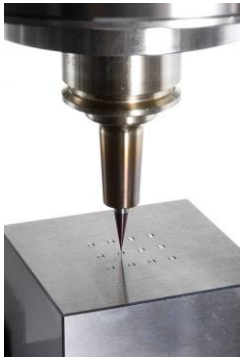
Integrated circuits mould (each figure dimension: 2,5 mm x 2,5 mm)
